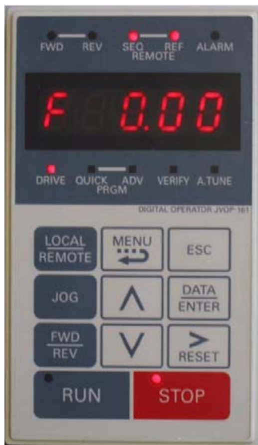
Fig 3.1 Digital Operator Component Names and Functions
