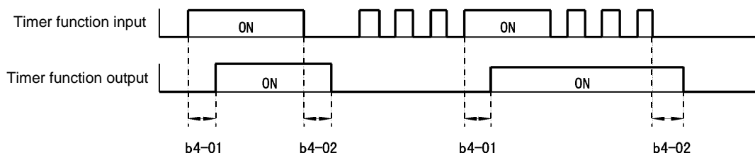
Fig 6.82 Timer Function Operation Example
