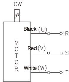
The direction of motor rotation is as viewed from the front shaft end of the motor
